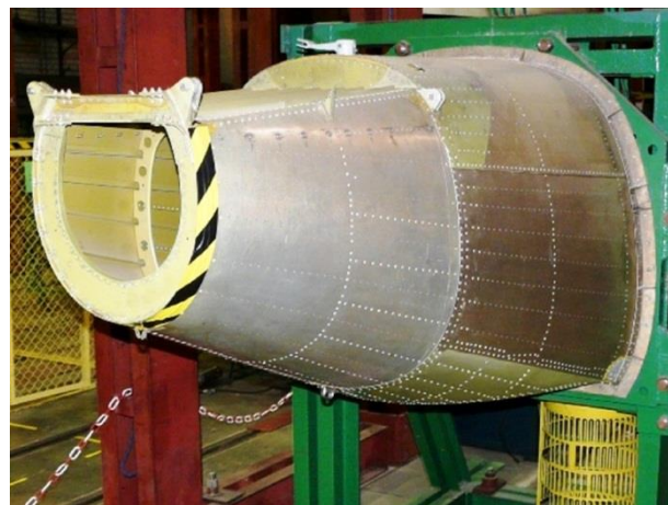
Figure 2 The rear fuselage for fatigue testing [3]
