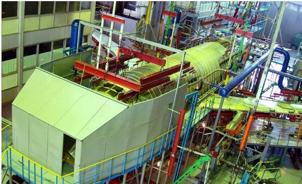
Figure 3 Fatigue testing of the entire aircraft [2]
