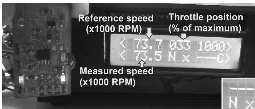
Figure 5 Generating RPM and throttle position PWM signals for the MARCEL turbojet controller
