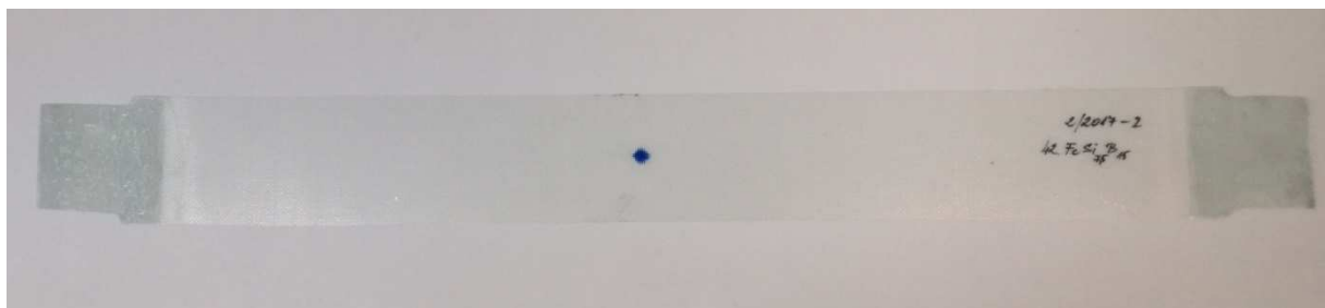
Figure 4 Glass fibre composite sample. Microwire position is marked by dot near the middle of the sample.
