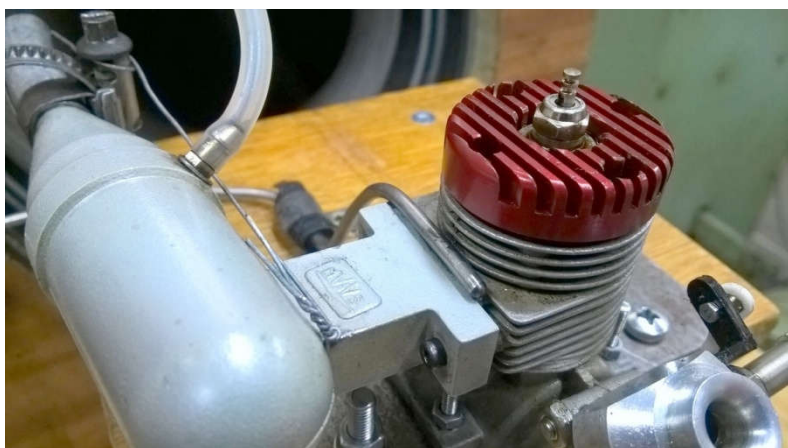
Figure 4 Place the thermocouple on the engine
