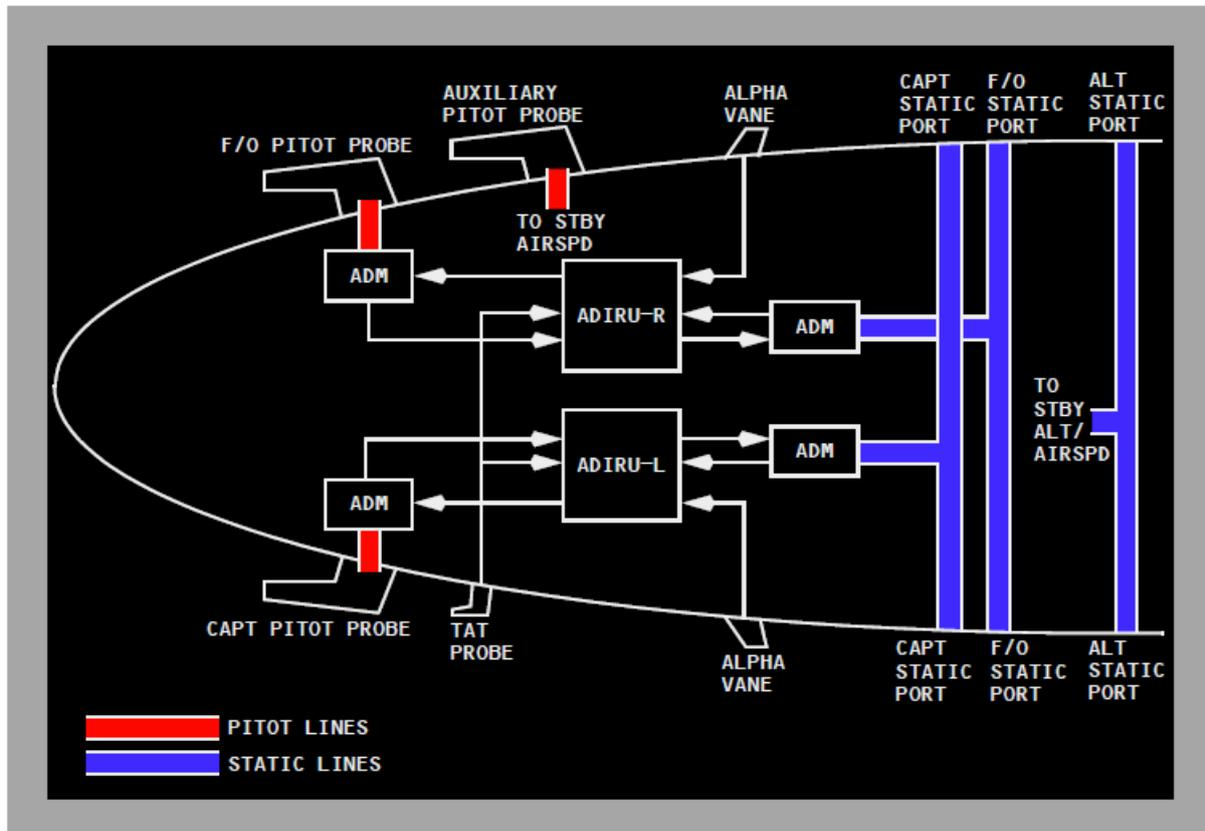
**Figure 4** Boeing 737 NG and MAX primary air data sensors with processing systems
