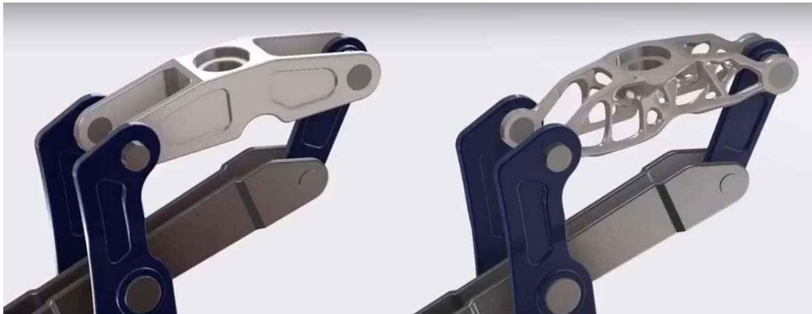
Figure 2 Example of using topological optimization [7]
