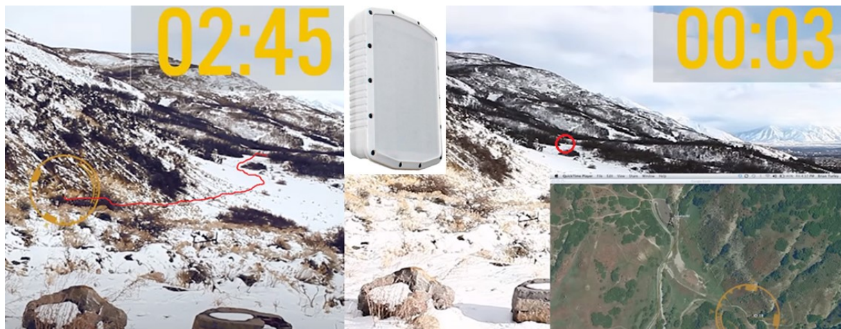
Figure 8 Comparison of camera and radar system intrusion detection
