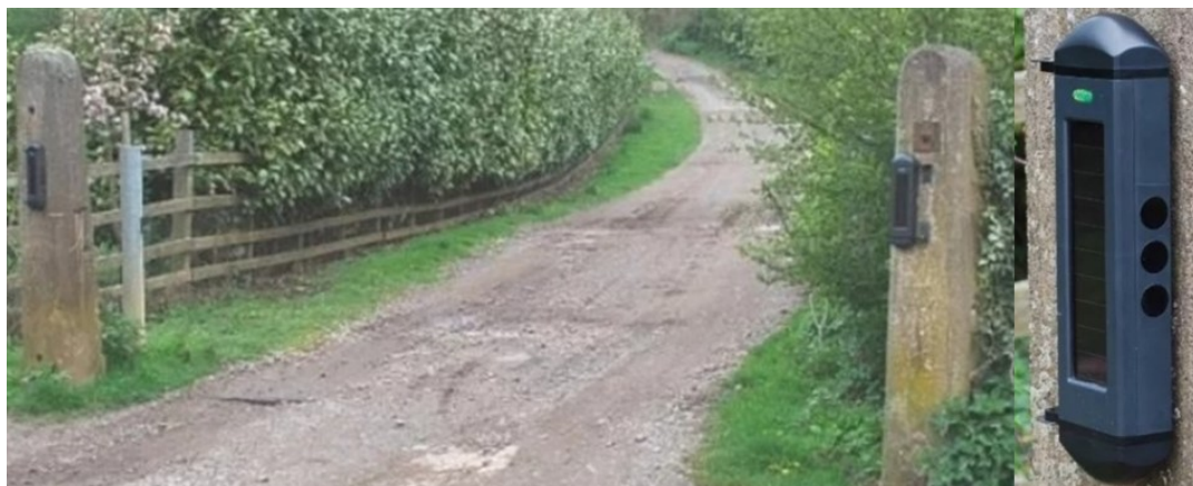
Figure 5 Example of using an IR barrier with a detailed view of an optoelectronic sensor / transmitter
