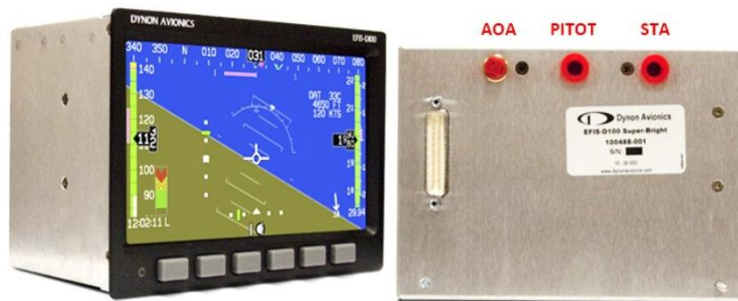
Figure 1 EFIS-D100 front and back view of the device [Author]
