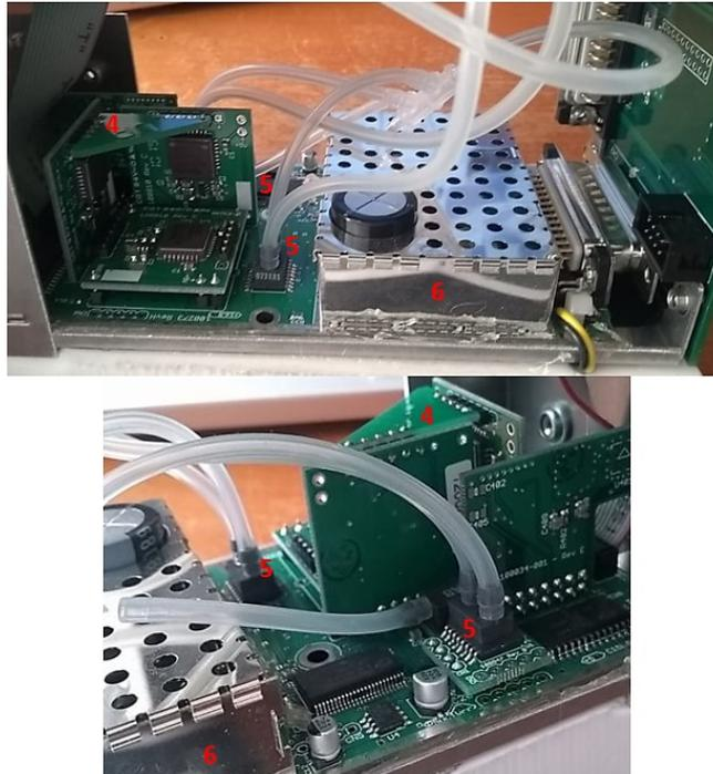
**Figure 3** View on the lower printed circuit board of the EFIS-D100 device [Author]
