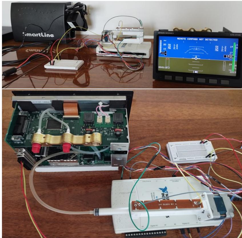
Figure 10 A simulation workplace controlling the change in flight height [Author]
