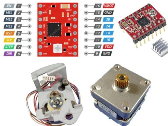
**Figure 4** EPSON EM-178 stepper motor and stepper control module engine A4988 [Author] [22] [23]
