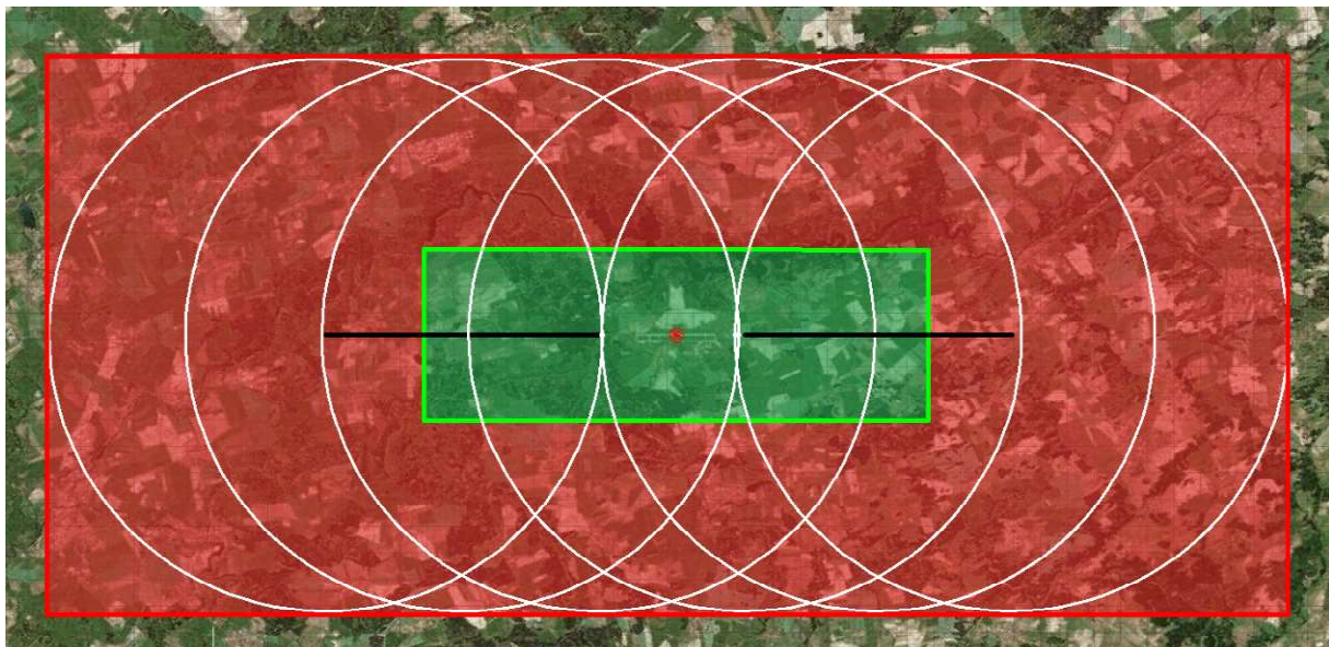
Figure 8 Satellite image of single RWY airport with marked circles with a radius of 7 NM forming a protective zone around the final approach tracks
