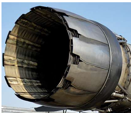
Figure 10 F110 all-mode adjustable supersonic engine output nozzle [9].
