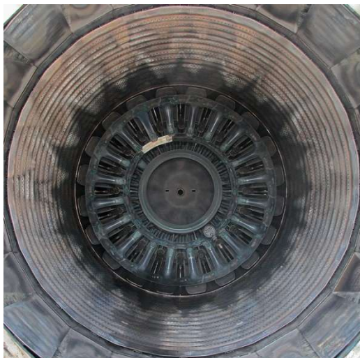
Figure 9 Afterburner combustion chamber of the F110-GE-129 turbofan engine [8].
