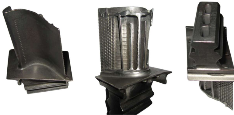
Figure 7 Cooled rotor blades of F110-GE-129 high pressure gas turbine engine
