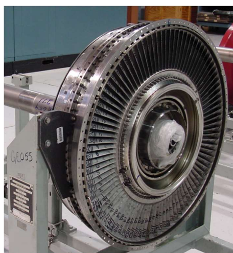
Figure 8 Disassembled low pressure gas turbine of engine F110-GE-129 node [6].
