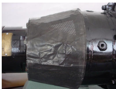
Figure 11 TV screen on the MPM-20 intake system
