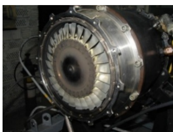
Figure 12 Damaged rotor blades of turbine
