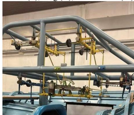
Fig. 9 Tunnel balances
