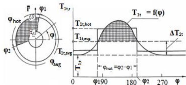
Fig. 1 Determination of thermal irregularities
