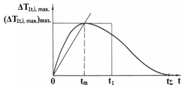
Fig. 2 Determination of thermal non-stationary parameters
