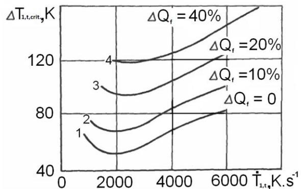
**Fig. 7 Function of  $\delta T_{1t,crit.}$  on  $\delta \dot{T}_{1t}$  where: 1 -  $Q_{fuel} = \text{const.}$ , 2 - rapid decrease of  $Q_{fuel}$  by 10%, 3 - rapid decrease  $Q_{fuel}$  by 20%, - rapid decrease  $Q_{fuel}$  by 40%**
