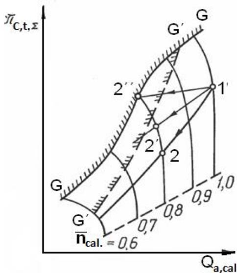
**Fig. 6 Effect of circumferential non-stacionarity of thermal field to the working point in compressor characteristic**
