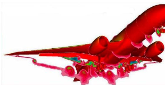
FIGURE 4: CFD SIMULATION OF AEROACOUSTICS [5]
