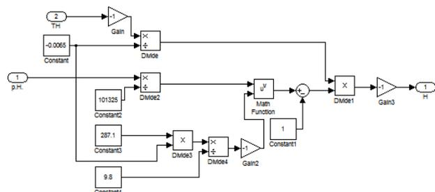
Picture 2 Model of simulating for barometric altimeter
