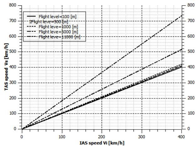
Picture 9 Graphic representation TAS speed and IAS speed in depending on flight level
