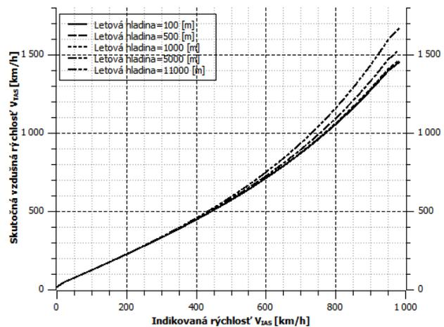
Picture 13 Graphic representation TAS speed and IAS speed in depending on flight level in compressible medium
