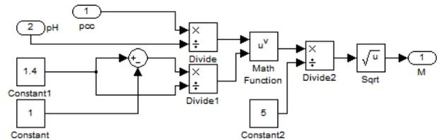
**Picture 15 Model of simulating Mach's number in supersonic zone**
