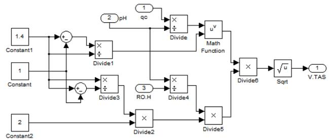
Pictre 12 Model of simulating TAS speed in compressible medium
