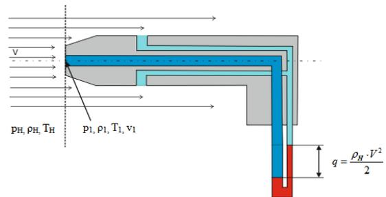
Picture 6 Pitot-static tube and formation dynamic pressure
