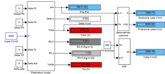
Picture 5 Model of barometric altimeter
