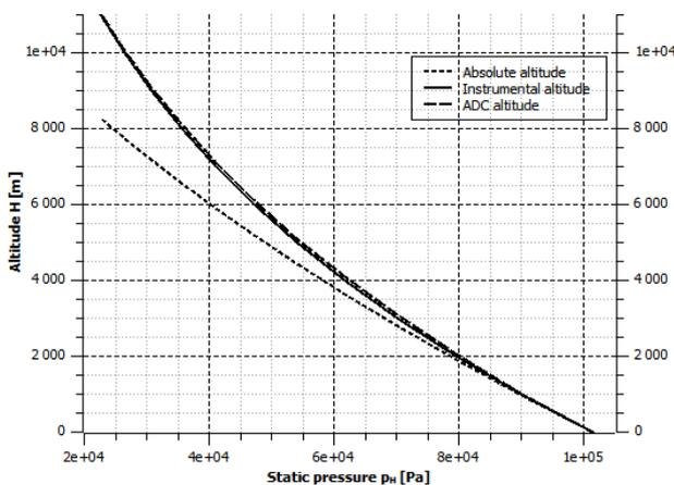
Picture 4 Graphic representation altitude of barometric altimeter and ADC
