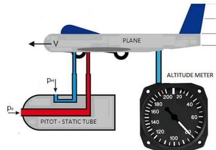
Picture 1 Altitude meter connect to Pitot-static tube
