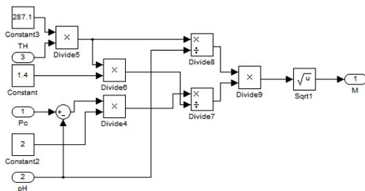
**Picture 14 Model of simulating Mach's number in subsonic zone**
