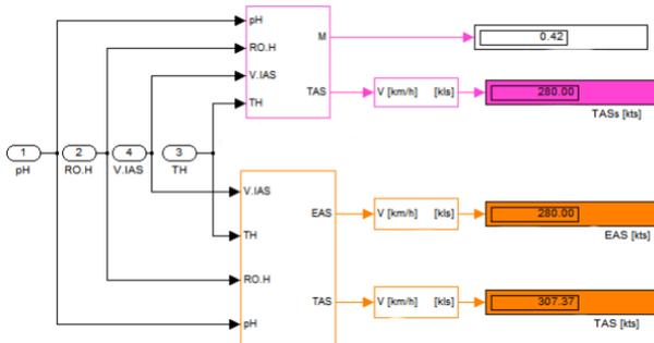
Picture 17 Model of speed meter
