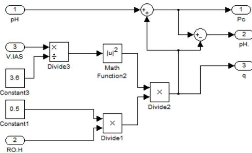
Picture 7 Model of simulating for dynamic pressure
