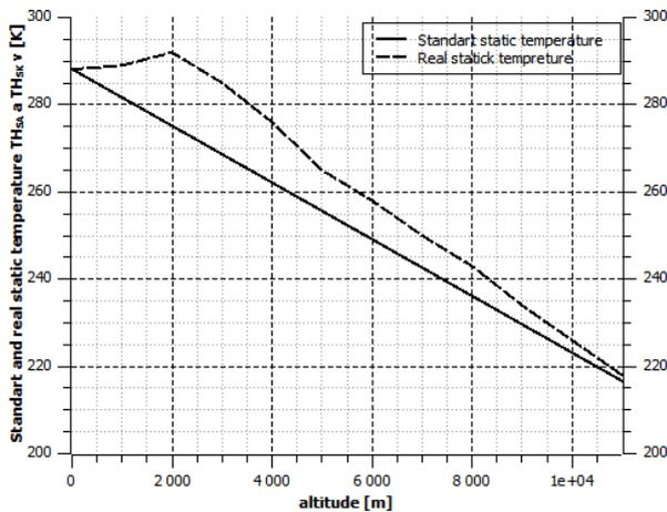
Picture 3 Graphic representation standart and real static temperature
