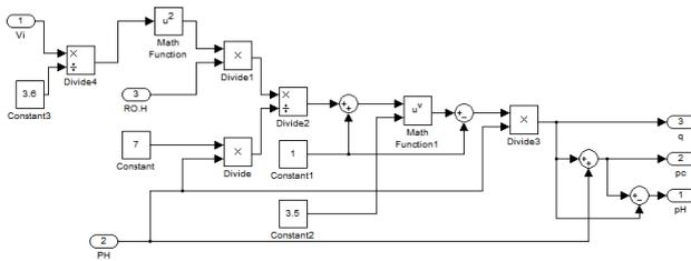
Picture 10 Model of simulating dynamic pressure in compressible medium
