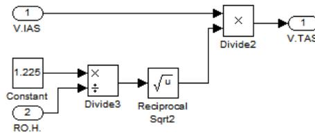
Picture 8 Model of simulating for TAS speed
