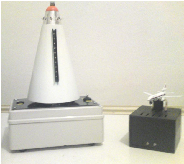
Fig. 8 Opto-electronic VOR/DVOR model
