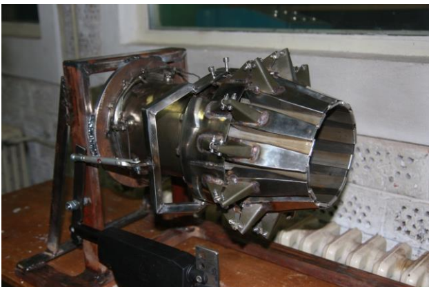
Fig. 2 MPM-20 nozzle on testing stand
