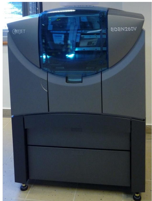
Figure 18. 3D printer used for model manufacturing 1
