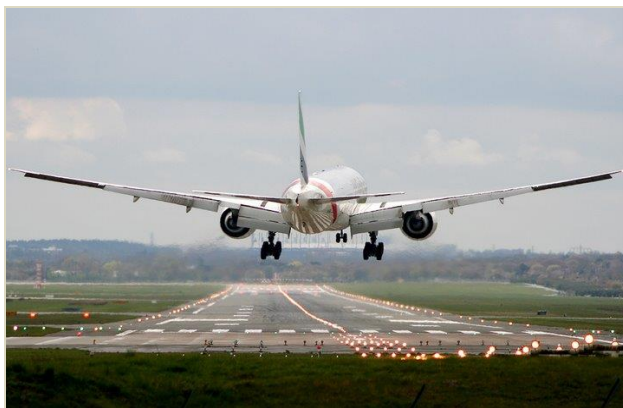
Fig. 5 Landing with a crosswind - course method
