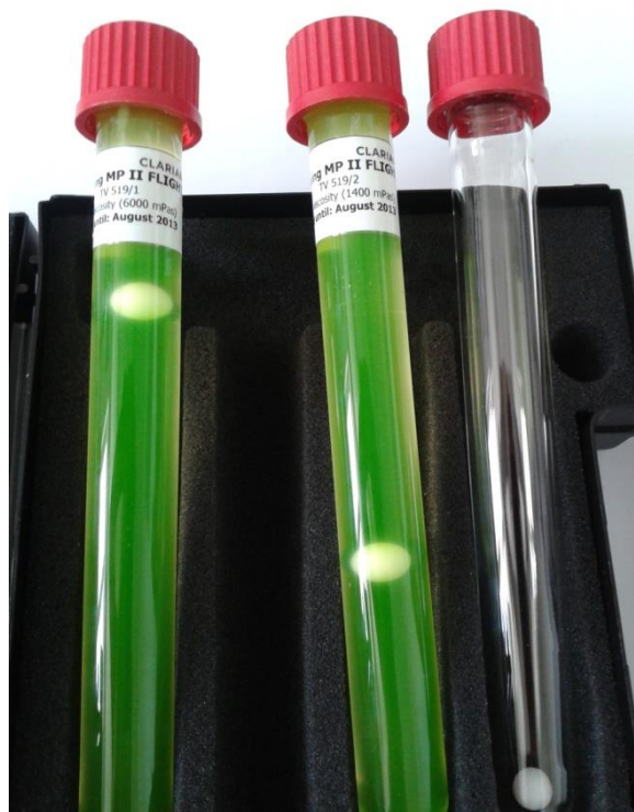
Figure 1 Safewing MP II FLIGHT - viscosity test
