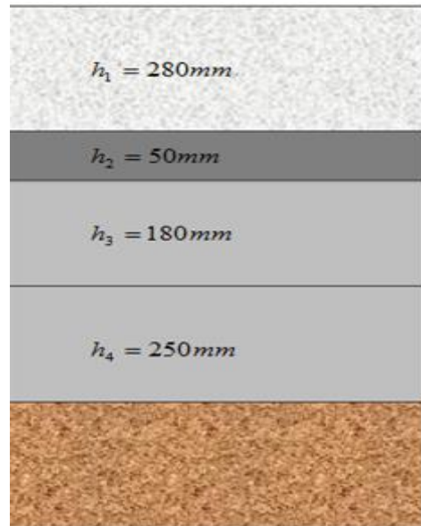
Figure 2. Proposal tracks CB construction of airport road
