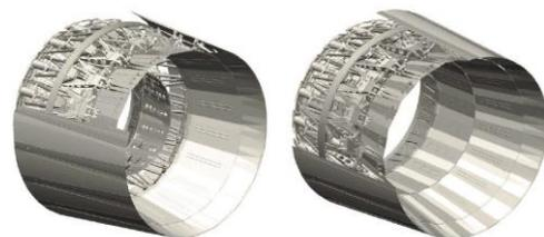
Figure no. 2 Adjustable nozzle with segments, by [5]
