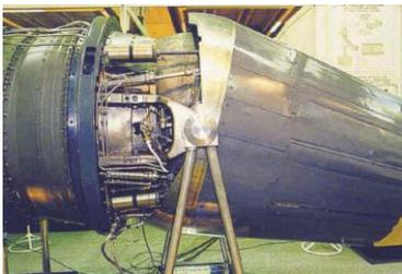
Figure no. 4 Axially symmetric nozzle with adjustable swivel hub, by [5]
