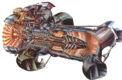
Figure no. 5 Engine Rolls-Royce Pegasus with 4 nozzles, by [0]
