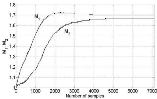
**Fig. 4, Learning process of multiplicative constants of x and y channel**
