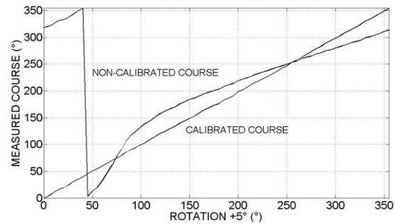
Fig. 11, Course calculated from measured and calibrated data
