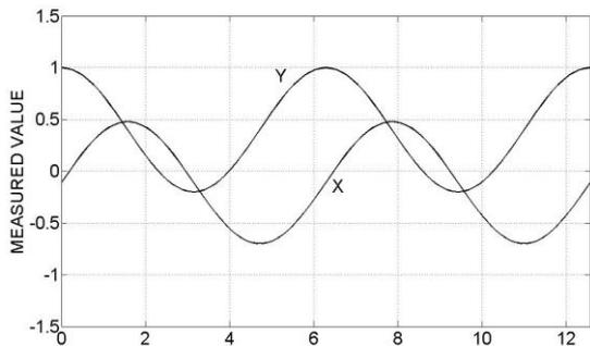
**Fig. 2, Time dependence of x and y sensors outputs while harmonic rotation**
