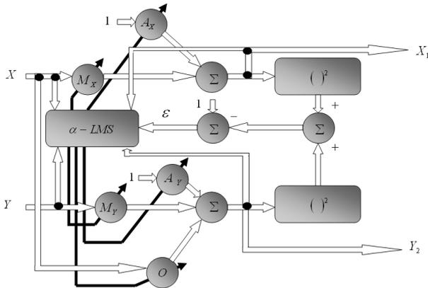
**Fig. 3, Neural network for multiplicative, additive and orthogonal error rejection**
