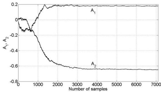
Fig. 9, Learning process of additive constant of channel x and y in real experiment
