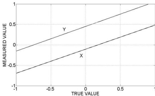
**Fig. 1, Transfer function of 2D sensor with additive, multiplicative and orthogonal error**
