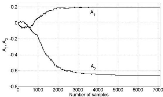
**Fig. 5, Learning process of additive constants of x and y channel**
