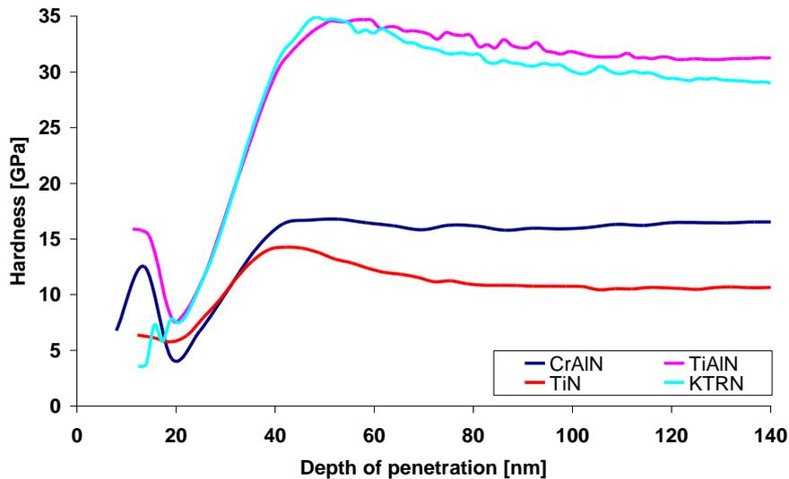
Figure 5 The nano-hardness of CrAlN, TiAlN, KTRN and TiN coatings
