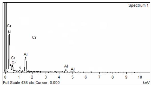
Figure 4 Brittle fracture (micrograph) and EDX spectrum of CrAlN coating on HSS Co 5 steel, thickness 1,2 μm.
