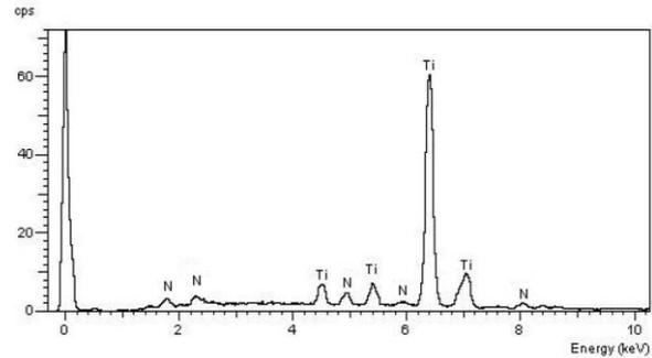
Figure 3 Brittle fracture (micrograph) and EDX spectrum of TiN coating on HSS Co 5 steel, thickness 2,1 μm.
