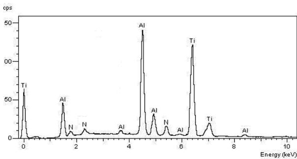
Figure 2 Brittle fracture (micrograph) and EDX spectrum of TiAlN coating on HSS Co 5 steel, thickness 1,6 μm.
