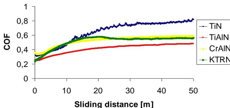
Figure 6 Coefficient of friction of CrAlN, TiN, TiAlN and KTRN coatings.
