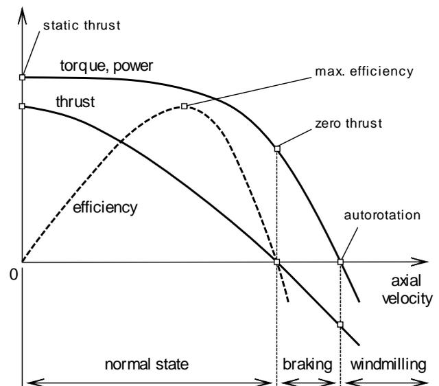
Figure 1. Aerodynamic performance of propeller
