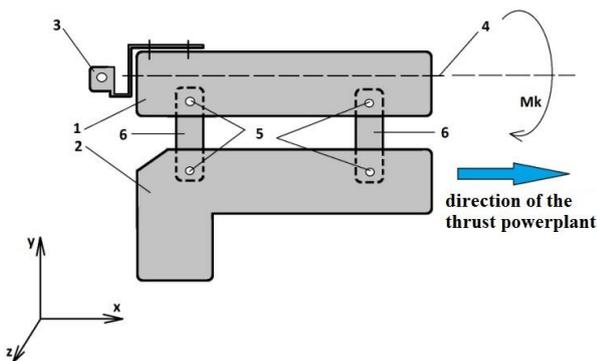
Figure 5. Cradle assembly with pantograph
