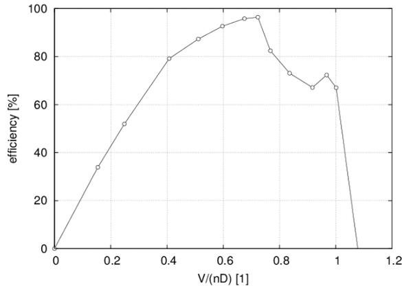
Figure 9. Measured propulsive efficiency at higher rotational speed
