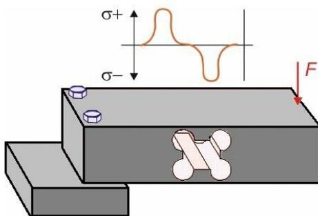
Figure 2. Cantilever deformation element for sensing of the normal force [5]
