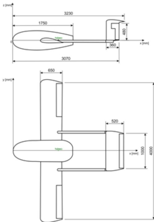
Fig.8 Proposed and calculated dimensions of the drone (UAV)
