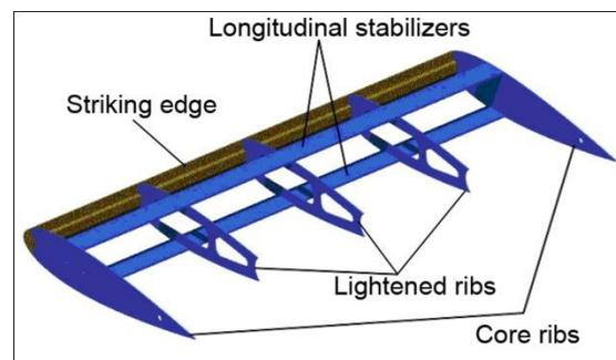
Fig. 6 Construction of horizontal tail surface
