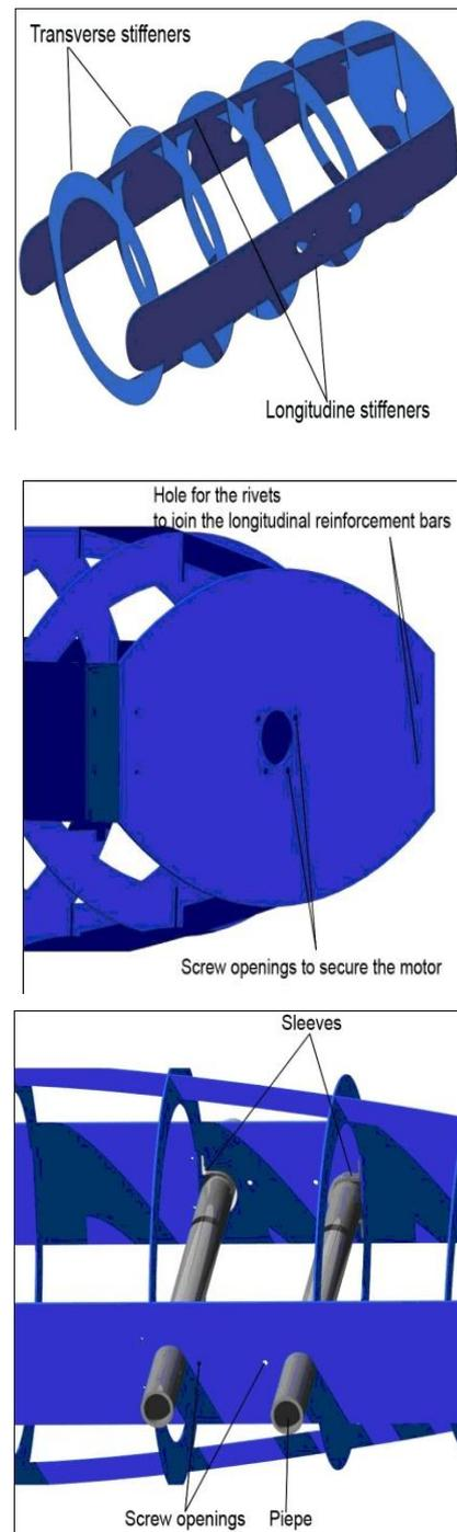
Fig. 2 Supporting structure of the fuselage, wings and engine mount
