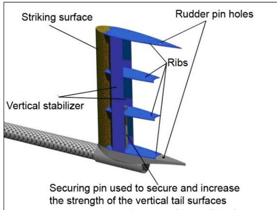
Fig. 5 Vertical tail surface construction
