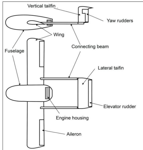
Fig. 1 Preliminary design of the aircraft shape
