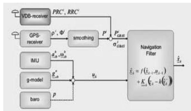
Figure 1 GBAS/INS system layout
