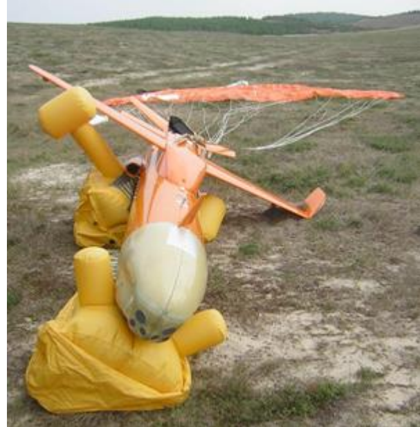
Figure 3. UAV parachute recovery system fitted with airbags [13]
