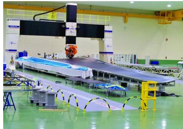
Fig. 7 Tapelaying machines for Airbus wings
