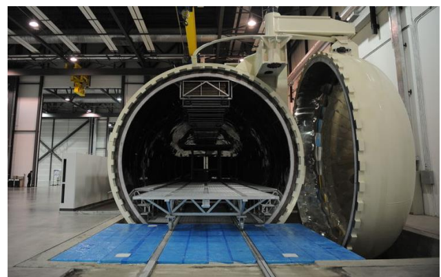
Fig. 8 Autoclave for wings and other large composites components
