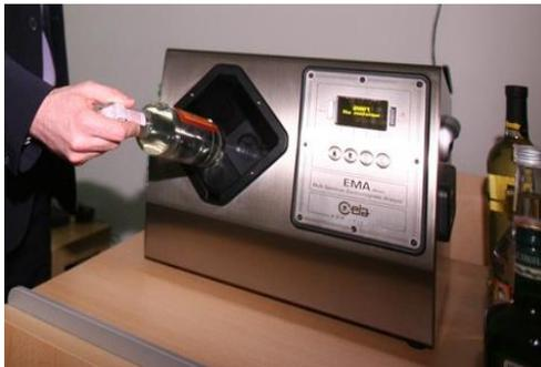
Fig.5. Scanner fluids
