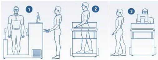
Fig.4. Procedure for passing shoe scanner
