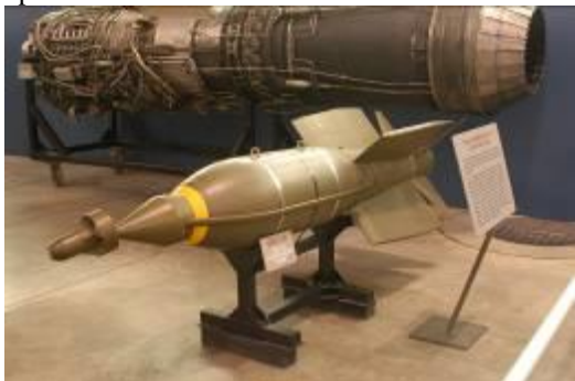
Illustration 1. BOLT-117 - the world's first laser-guided bomb (750 lbs).
