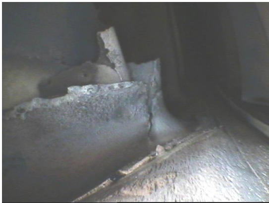
Fig. 14 Fractured guide vane of the low pressure gas turbine on the RD-33 engine (photo Martin Schmidt)
