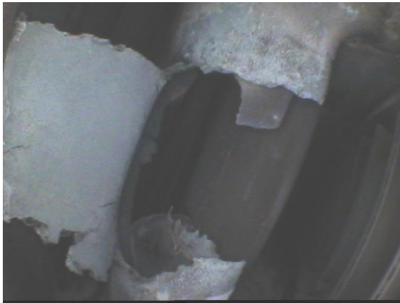
Fig. 17 An open guide vane of the low pressure gas turbine on the RD-33 engine (photo Martin Schmidt)
