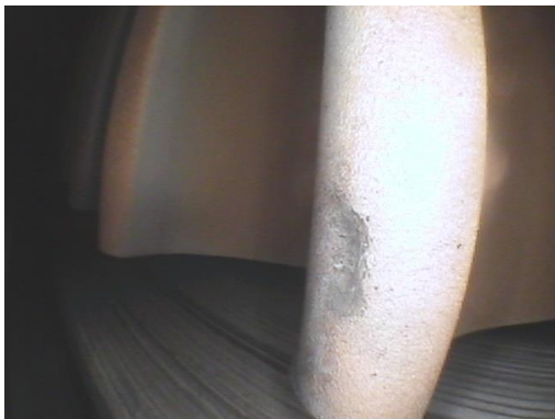
Fig. 10 Deformation on the surface of the rotor blade leading edge of the high pressure gas turbine (photo Martin Schmidt)
