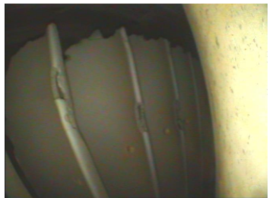
Fig. 16 Mechanically damaged rotor blades on the low pressure gas turbine of the RD-33 engine (photo Martin Schmidt)
