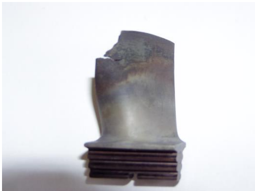
Fig. 9 Detail of the destroyed rotor blade, part of the MPM-20 experimental jet engine as a result of thermal and mechanical damage (photo Marián Hocko)
