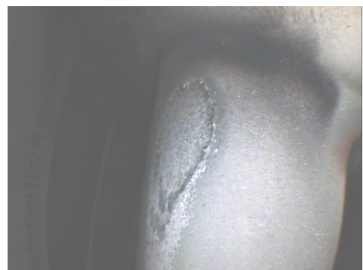
Fig. 6 Material cutting (burn-out) on the guide vanes in the guiding duct of the low pressure gas turbine of the RD-33 engine (photo Martin Schmidt)
