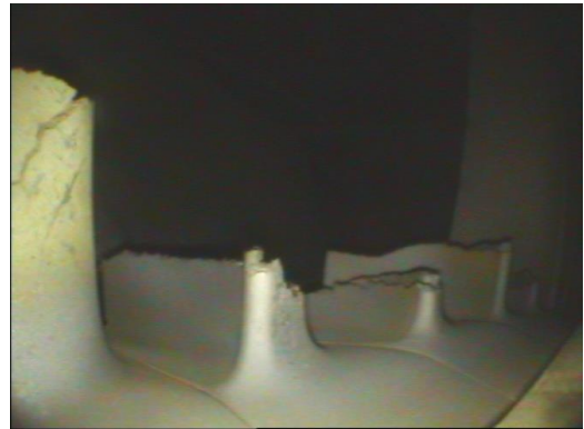
Fig. 15 Broken rotor blades of the low pressure gas turbine on the RD-33 engine (foto Martin Schmidt)
