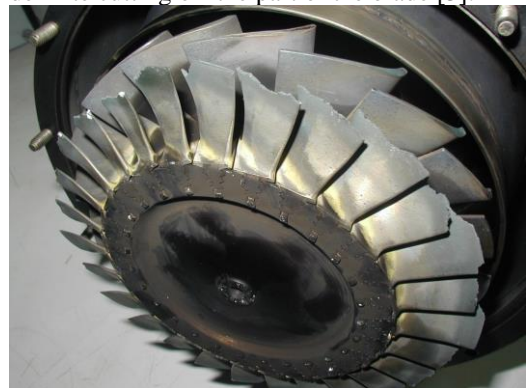
Fig. 8 Destroyed rotor blades of the gas turbine on the MPM-20 experimental jet-engine as a result of thermal and mechanical damage (photo Marián Hocko)
