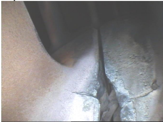
Fig.7 Material cutting (burn-out) in the area of contact with the sectors of guiding vanes (photo Martin Schmidt)
