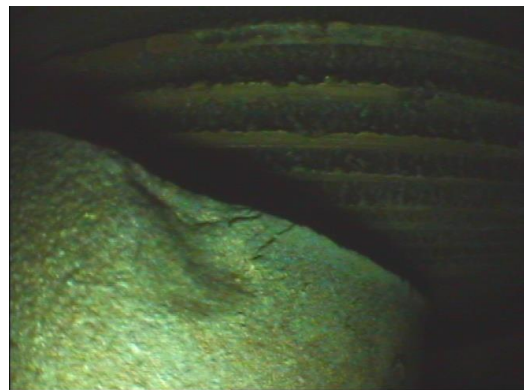
Fig. 12 Crack and collapse of the rotor blade on the high pressure gas turbine of the RD-33 engine (photo Martin Schmidt)
