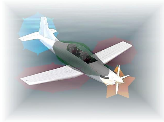
Figure 6: Calculated zone of impact [7]
