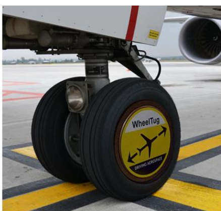
Fig. 9 The WheelTug system
