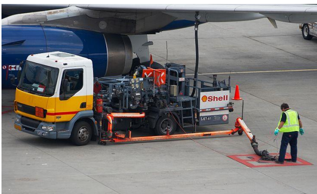
Fig. 4 Refuelling of aircraft from hydrant by dispenser
