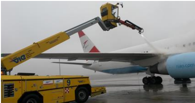
Fig. 7 De-icing of aircraft
