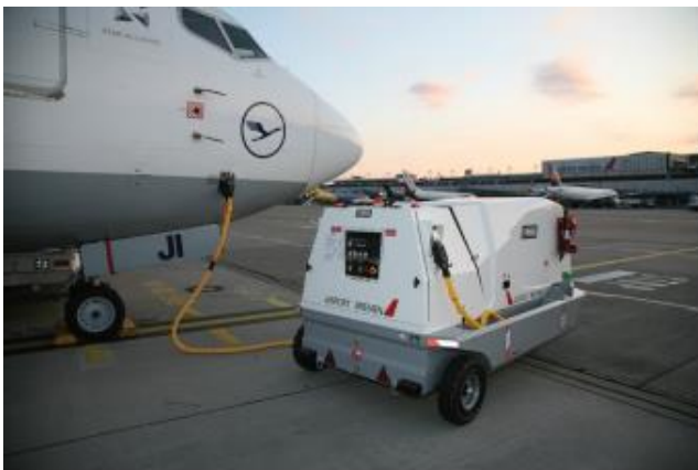
Fig. 3 External power supply
