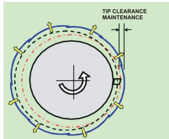
Fig. 11 Rub-avoidance ACC system
