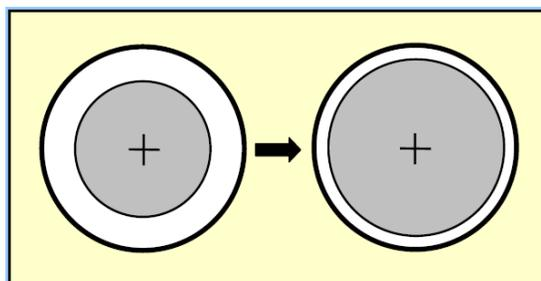
Fig. 1 Symmetrical changes of tip clearance
