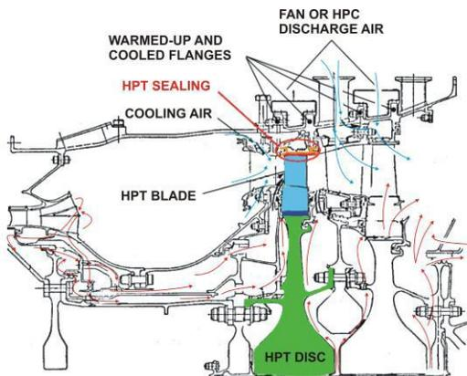
Fig. 7 Active thermal clearance control system
