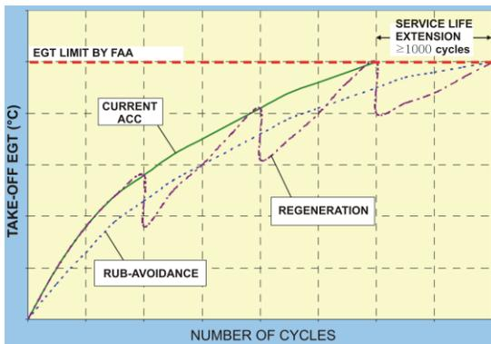
Fig. 13 Effect of rub-avoidance and regeneration ACC systems on take-off EGT [1, 2]
