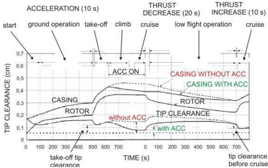
Fig. 4 Tip clearance change of HPT during flight phases
