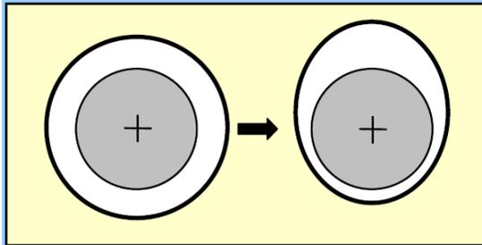
Fig. 2 Asymmetrical changes of tip clearance
