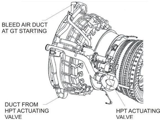
Fig. 9 HPT clearance control arrangement of CFM56
