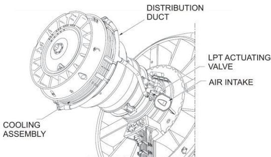
Fig. 10 LPT clearance control arrangement of CFM56
