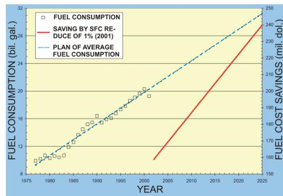
Fig. 6 History and schedule of fuel consumption and costs saving at reduction of SFC by 1%
