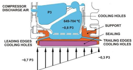
Fig. 5 Axial pressure layout in HPT casing
