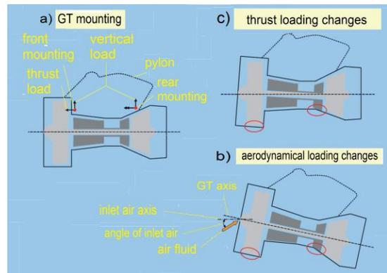
Fig. 3 a) GT mounting; b) Tip clearance change caused by aerodynamically load; c) Tip clearance change caused by thrust load
