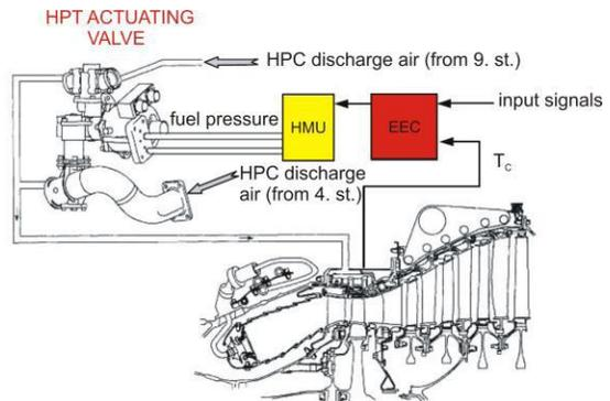
Fig. 8 HPT clearance control of CFM56
