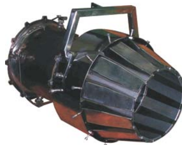
Fig. 1 Output control system for MPM20 engine with variable output section
