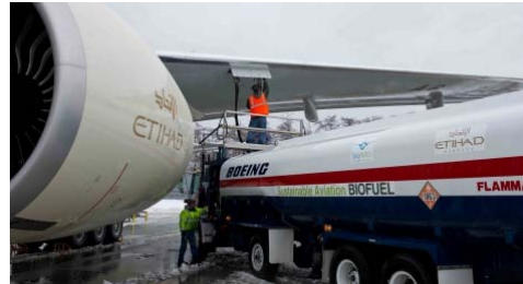
Figure 5. Etihad new Boeing 777-300ER tanking biofuel mixture prior to departure from Paine Field
