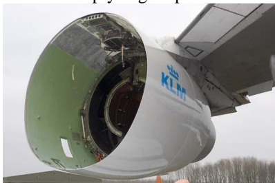
Fig. 5 GE-CF6 aircraft engine pod from Boeing 747 [7]
