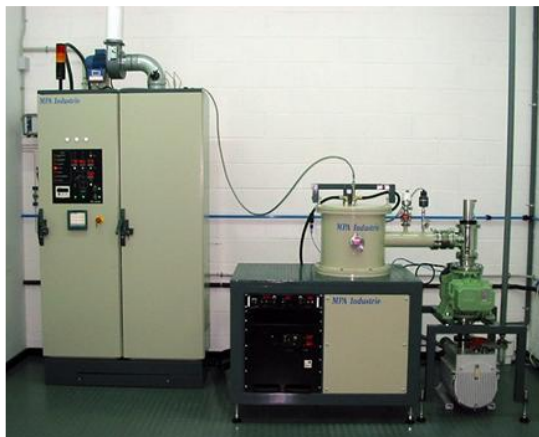
picture 5 system of coating by CVD [6]
