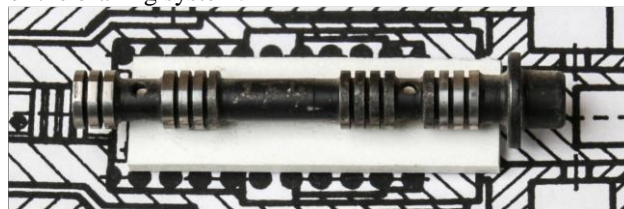
picture 7 differential valve with chrome coating
