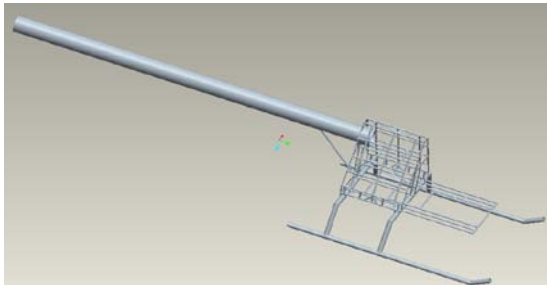
Fig. 2 Model of bearing PSS of helicopter designed in Pro Engineer Wildfire 4.0.
