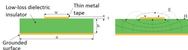
Figure 1. A microstrip waveguide
