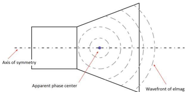
Figure 11. Plan view of the horn antenna
