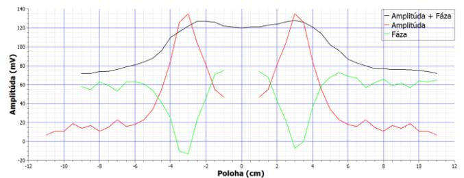
Figure 13. Amplitude and phase on the horn antenna
