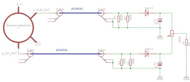
Figure 10. Functional interconnection circuit
