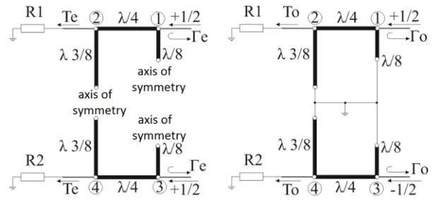
Figure 4. Equivalent circuit of a coupler
