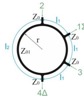
Figure 5. Principle of a circular mixer
