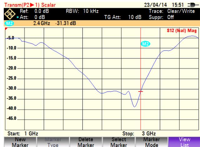
Figure 8. Transfer characteristic  $S_{14}$
