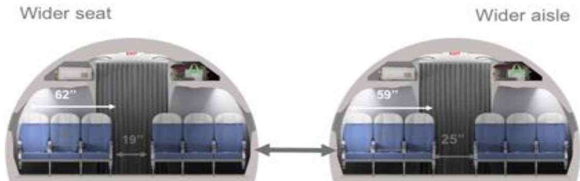
Fig. 1.: Cross-section of an Airbus A320 line body and options for seat configurations (Source: Airbus)
