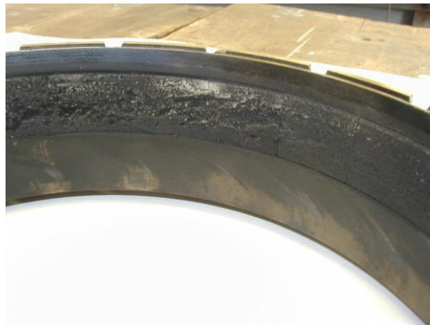
Figure 11 Burned sealant in the body of the gas turbine rotor blades
