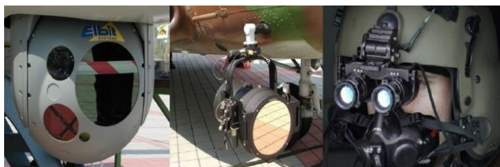
Figure.10 Termovision and a television camera, a search searchlight and night vision of the pilot of the helicopter
