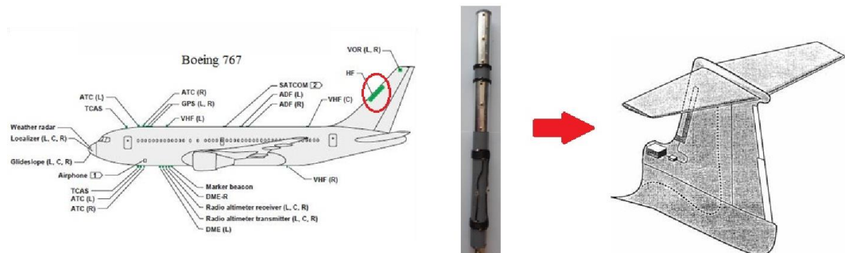
Figure 5 EH antenna for HF radio communication
