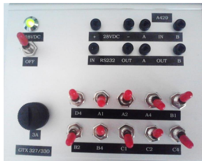
Figure. 4 Control unit for avionics check device
