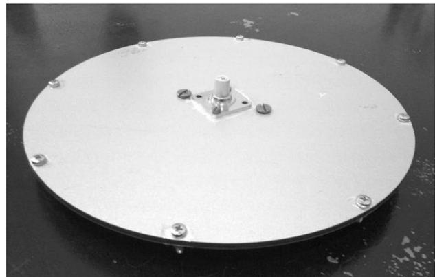
**Fig 2** Circular ground plane with monopole antenna
