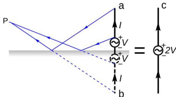
**Fig 1** Monopole antenna over a ground plane [2]
