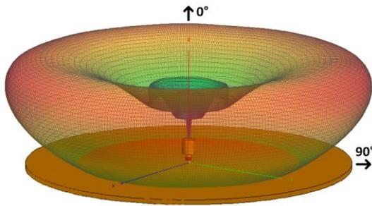
**Fig 3** Simulated radiation pattern in 3D for 6GHz
