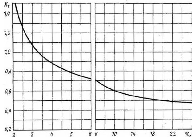
Fig.2 Dependency of coefficient K<sub>1</sub> on overall pressure ratio
