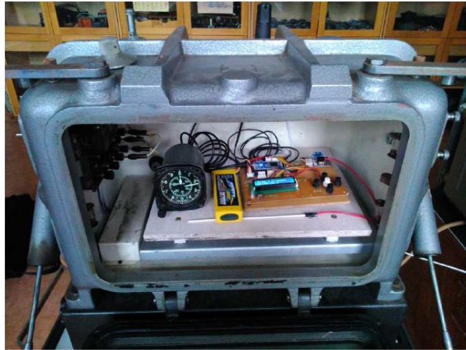
Figure 3 Testing of student designed MEMS aerometric system for small aircraft in a pressure chamber [6].
