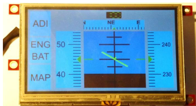
Figure 4 An example of student designed simple EFIS system with variety of visual representation modes of flight and navigation data [2].
