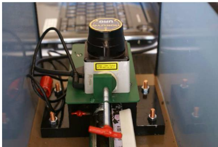
Figure 8 Stand device for laser distance measuring [11].
